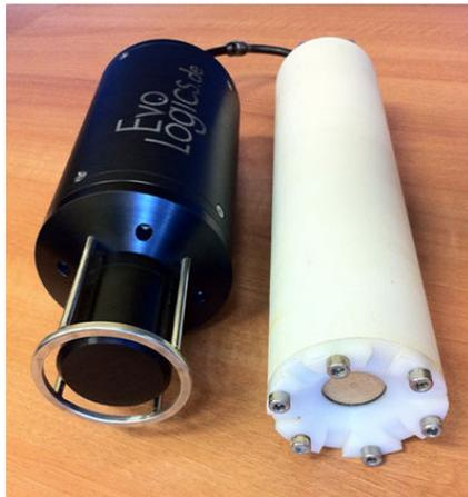
(a) CO2Probe and acoustic modem.
