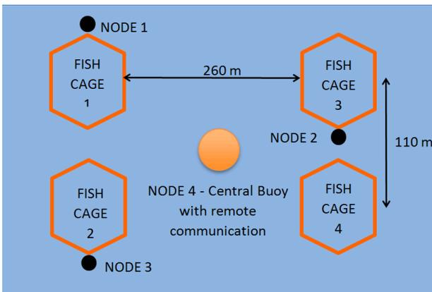
Figure 7: Deployed topology.
